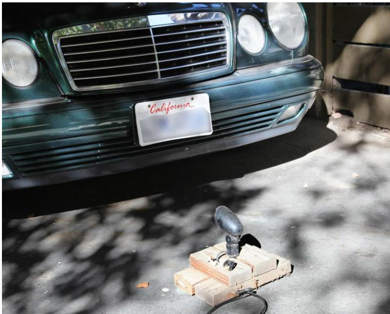
In this case I used the proper wire that is sold in hardware stores for lawn-lighting purposes. It is heavy guage (less loss on low voltage systems) and the insulation is designed for outdoor use.
